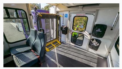
Interior of LINK vehicle showing accessible lift.
