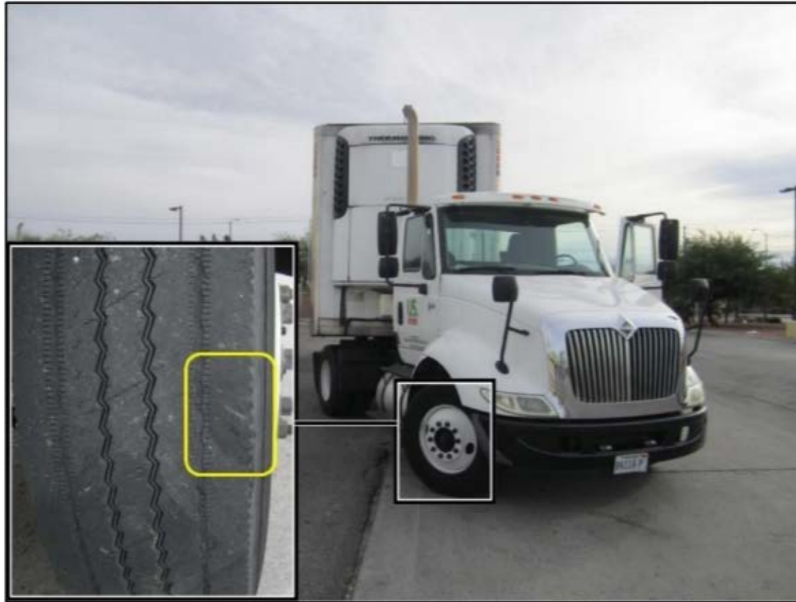
Figure 3. Truck-tractor after collision, with inset showing damage to right front tire (photo taken 4 days after collision).
